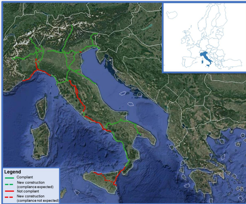
Figure 24: Status of compliance of the Italian TEN-T core network corridors to P400 in 2030
