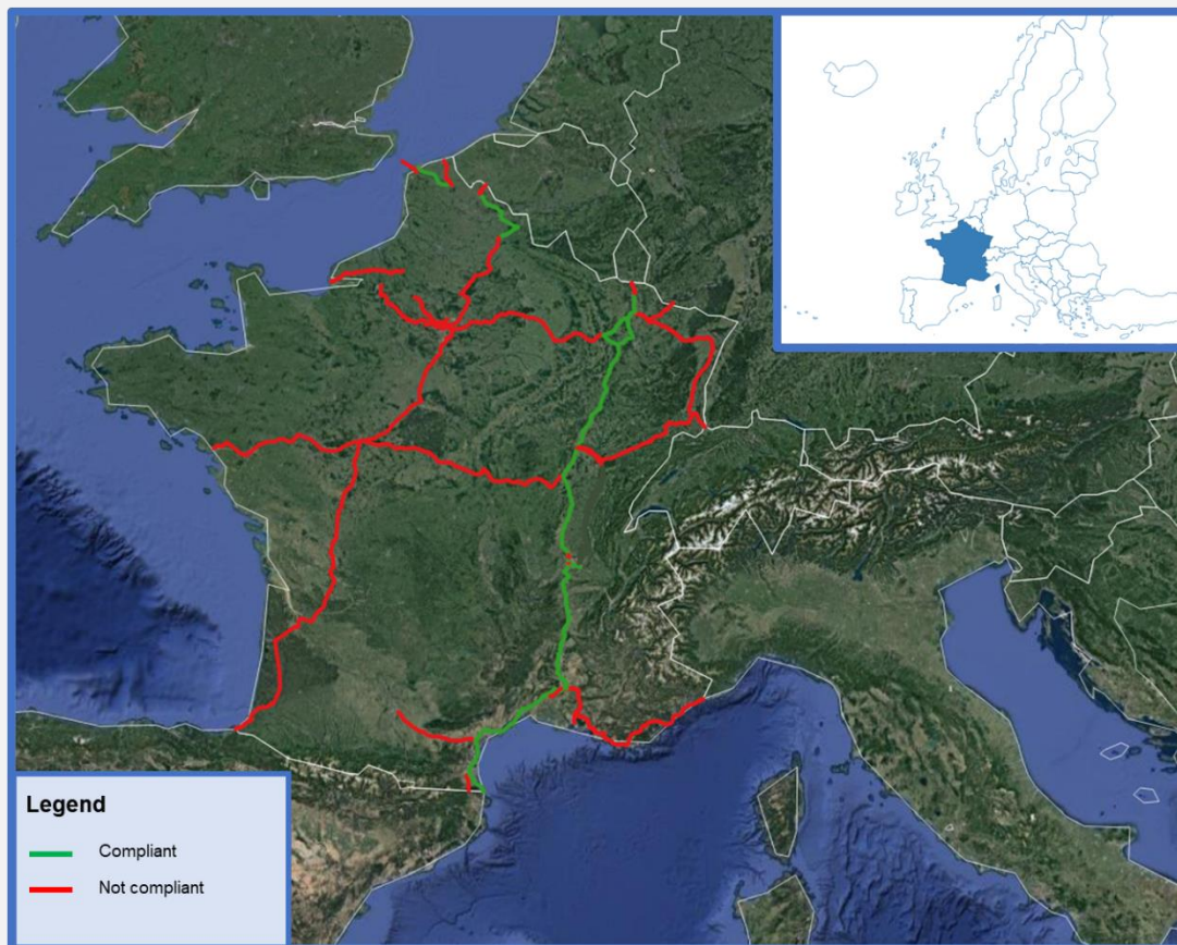
Figure 21: Status of compliance of the French TEN-T core network corridors to P400 in 2021 (SNCF reseau database)
