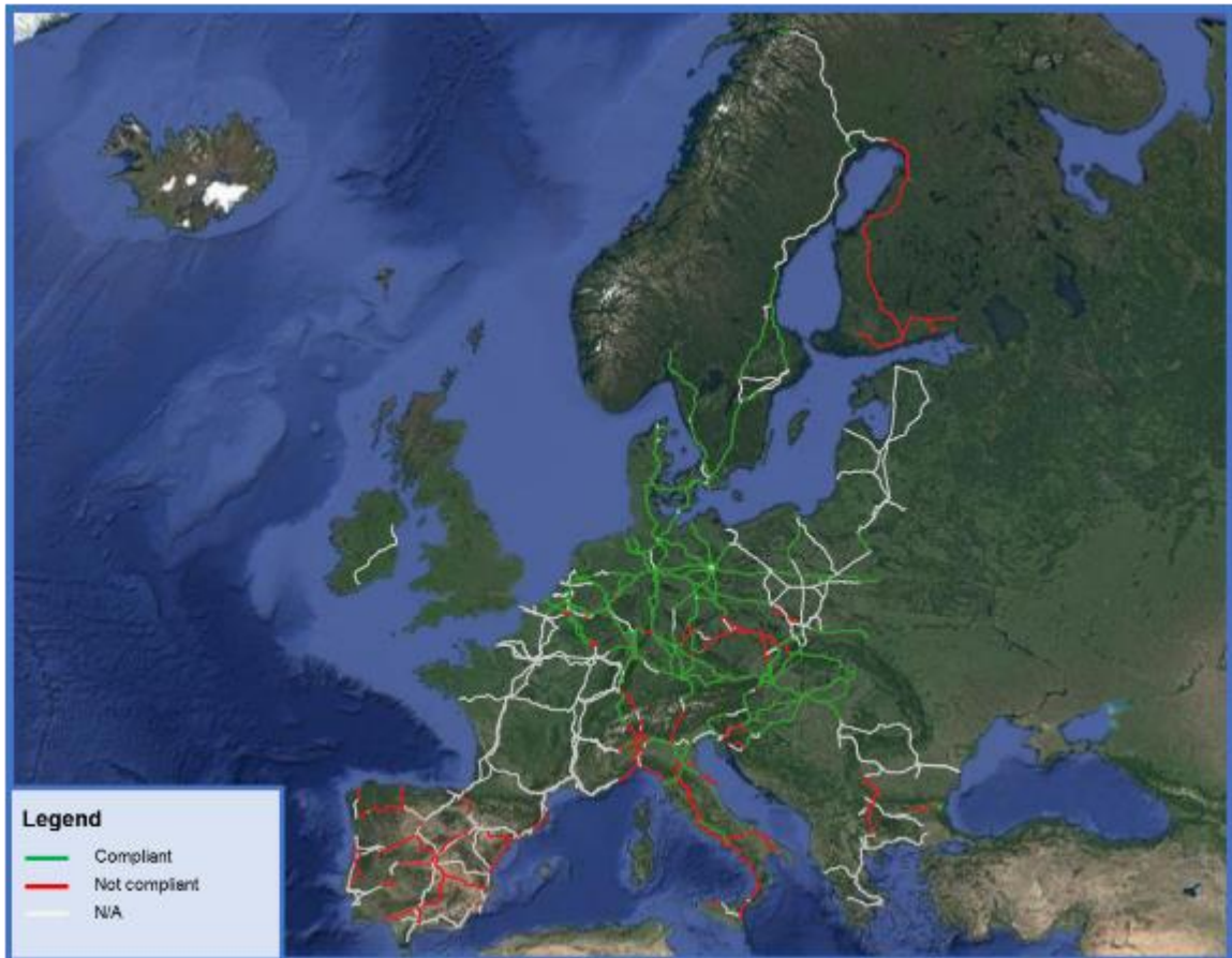
Figure 14: Status of compliance of the TEN-T core network corridors to P400, TENtec database
