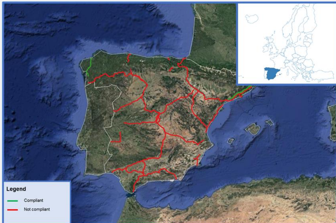
Figure 27: Status of compliance of the Spanish TEN-T core network corridors to P400 in 2021 (ADIF database)
