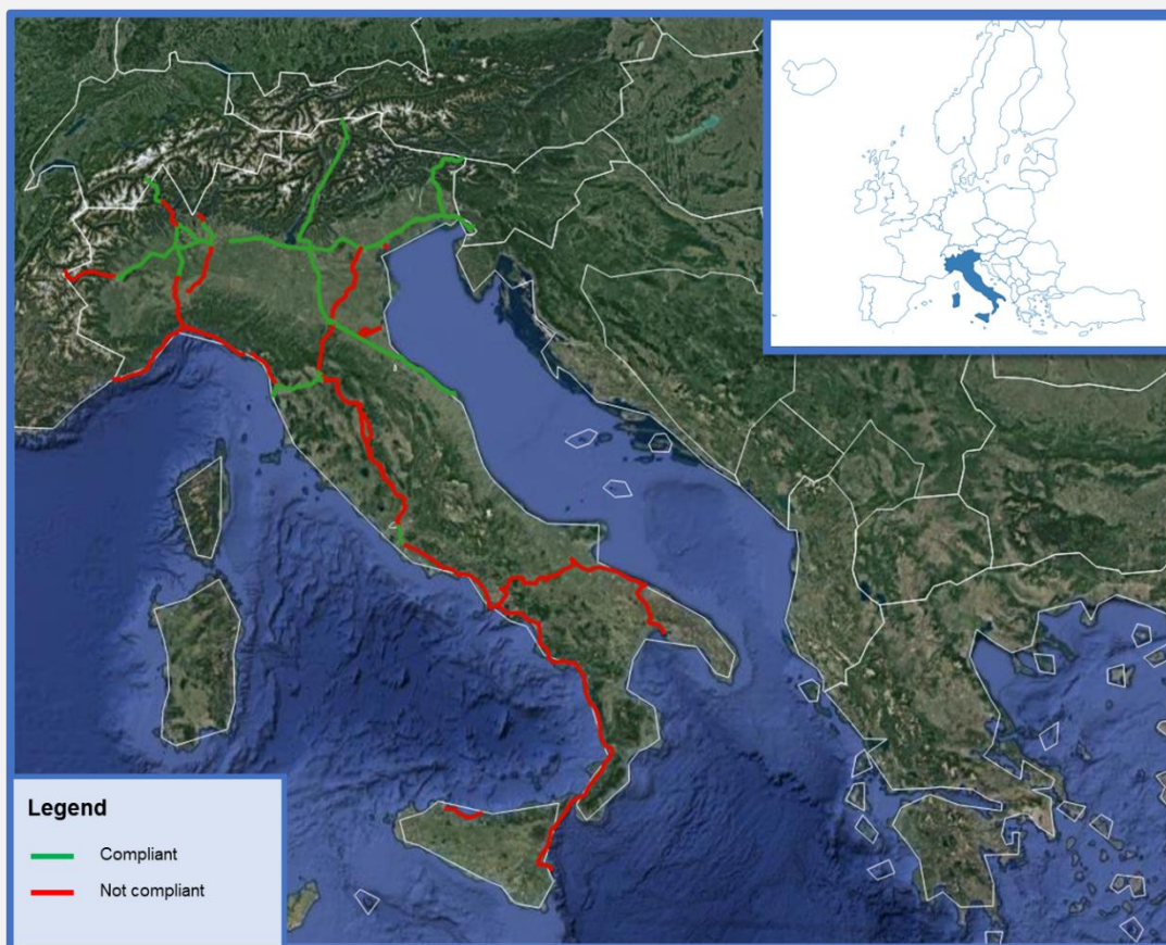
Figure 23: Status of compliance of the Italian TEN-T core network corridors to P400 in 2021 (RFI database)
